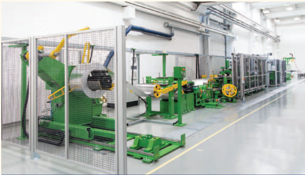
The key processes forming, welding and extrusion from one source. Rosendahl Nextrom's RH-W production line.
